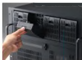
Four hot-swap cooling fans with filter
