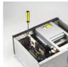
User-friendly mechanical design for installing an add-on card
