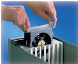
Hot-swappable cooling fan module contains one 53 CFM cooling fans
